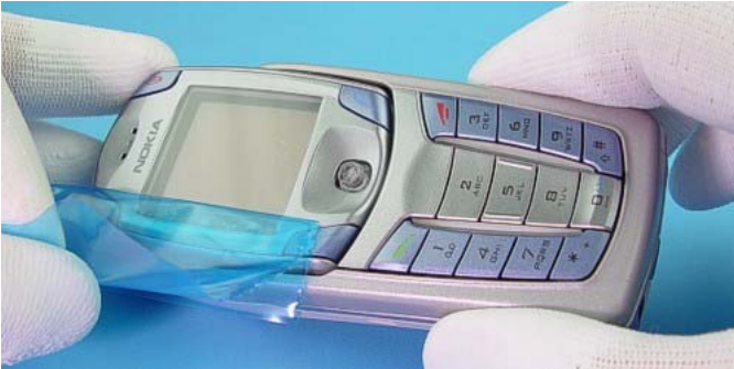
Check the condition of Window Protect the Window with a film.
