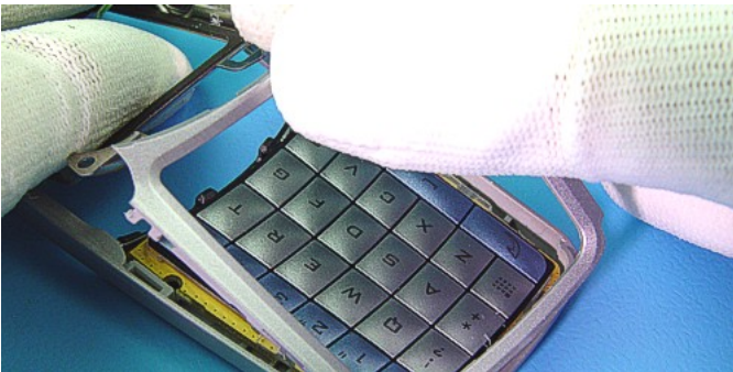
Now, Qwerty Frame is loose. Always use a new Frame during assembly
