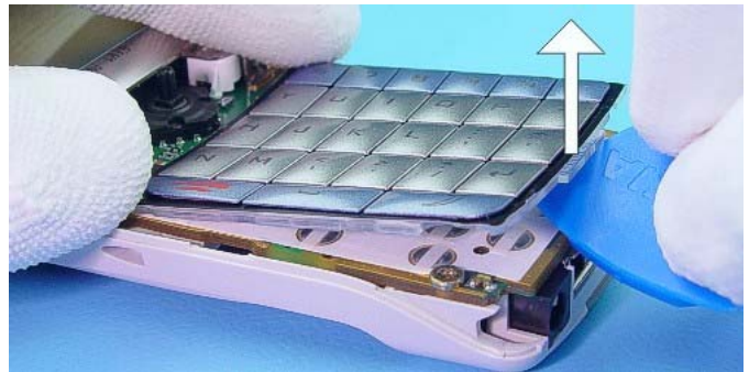
The Bottom side of the Keymat is glued to the Keydome therefore move up the Keymat with SRT-6 carefully. Mind the underneath LEDs.
