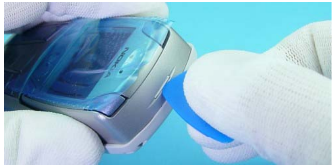
To remove the A-Cover, release the clip first by using SRT-6.
