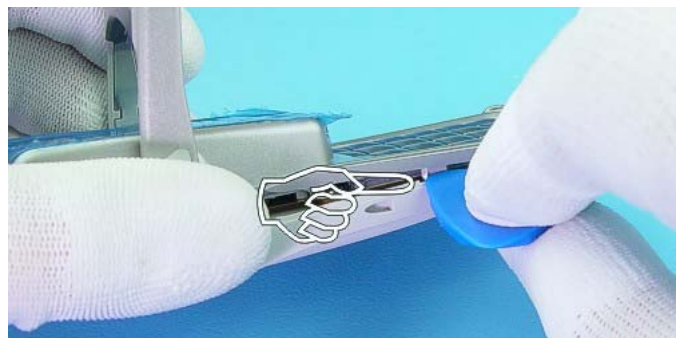
Lift the topside of the A-Cover a bit and open the bottom clip.
