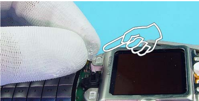
Remove the Joystick Button.
