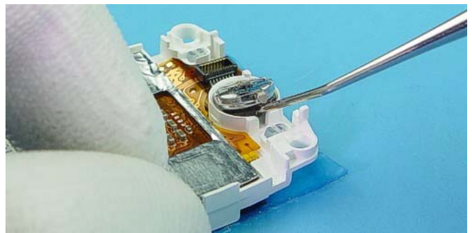
The Earpiece is attached with double-sided adhesive Foam Tape. Always use a new tape when mounting the Earpiece.
