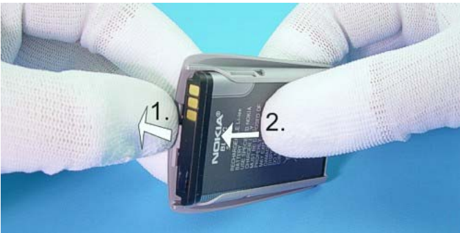
Remove Battery from Battery Cover as shown.
