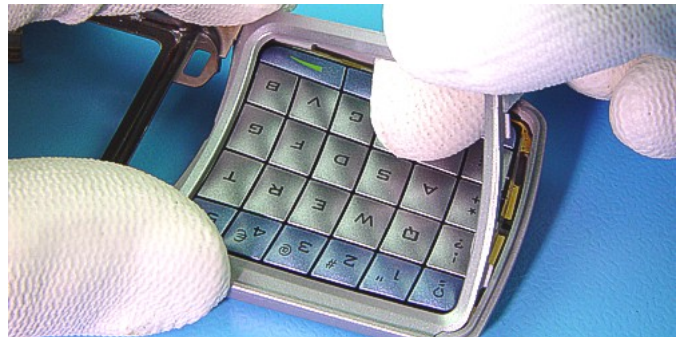
Use fingers to grip the Qwerty Frame and release the leaving snaps.
