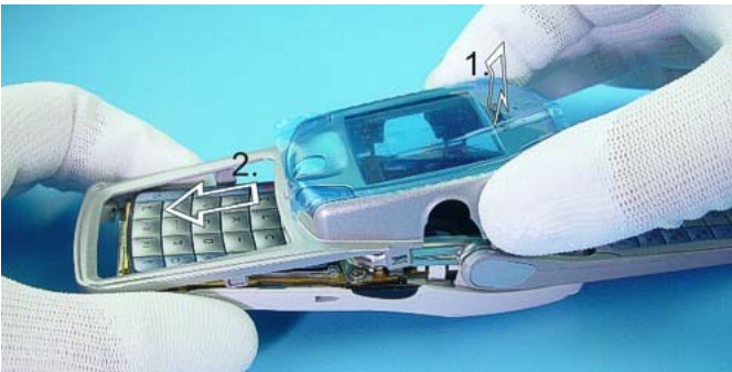
First lift the topside of the A-Cover then move the A-Cover forward.
