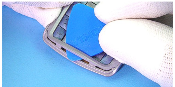
Carefully place SRT-6 between Qwerty Frame and Flip.
